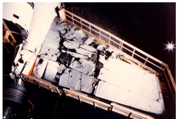
Fig. 2. The example of uncontained engine debris failure which happened with DC-10-10 19 th June 1989
