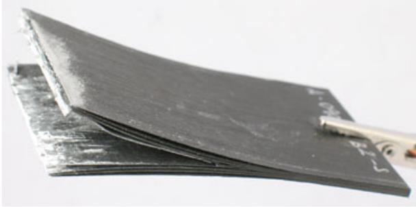
Fig. 4 Crushed flat specimen
