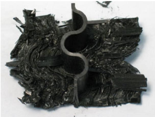
Fig. 5 Crushed self-supporting specimen
