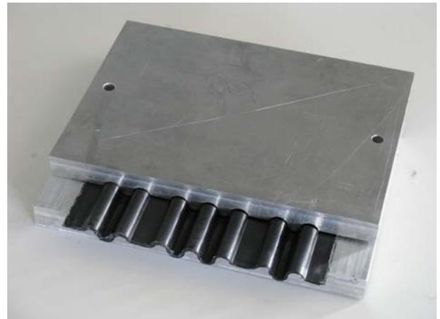
**Fig. 9** Mold for self-supporting specimen with carbon fiber plate
