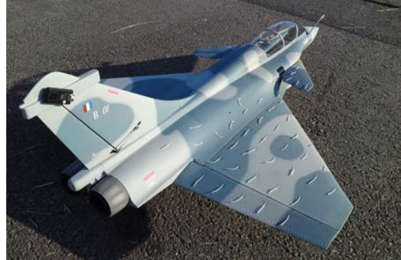
Fig. 3. Test setup with camera and wool tufts.
