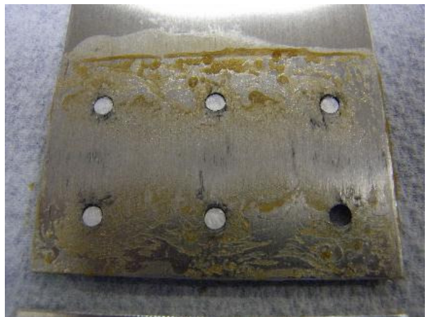
Fig. 4. LPS-3 treated specimen tested at 11.3kN.
