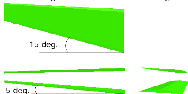
Fig. 6 Orthographic views of wing model used for validation
