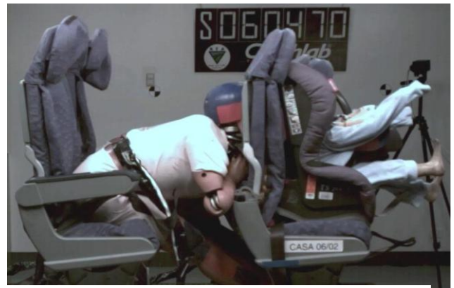
Figure 1 Rear passenger impact with child restraint system installed [2].
