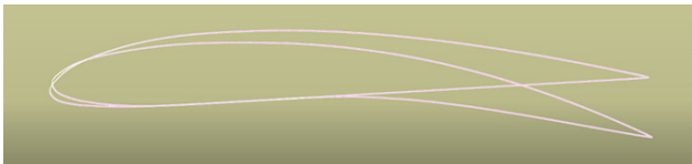
Fig. 3 Morphing of Wing Panel When the SMA Wires are Fully Actuated
