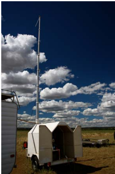
Figure 3: Self erecting mast on site with directional antenna installed
