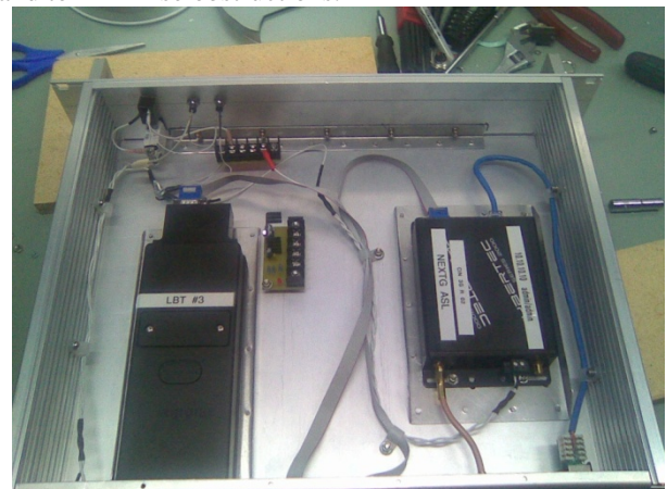
Fig 2. Aircraft Communications Rack with installed Next GTM Network modem and Iridium LBT modem
