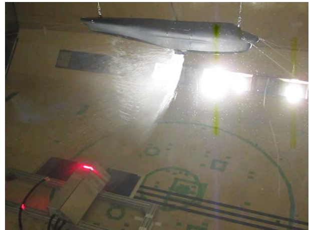
Fig. 12. Shadow imaging measurement for water dropping in the wind tunnel.
