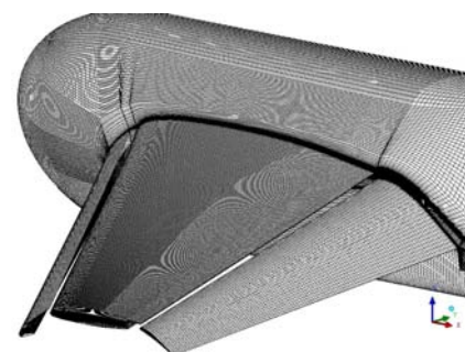
Fig. 6 Surface mesh for configuration one (Hexahedral Mesh).
