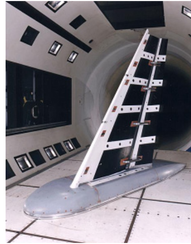
Fig. 4 Trapezoidal wing in the wind tunnel test section.
