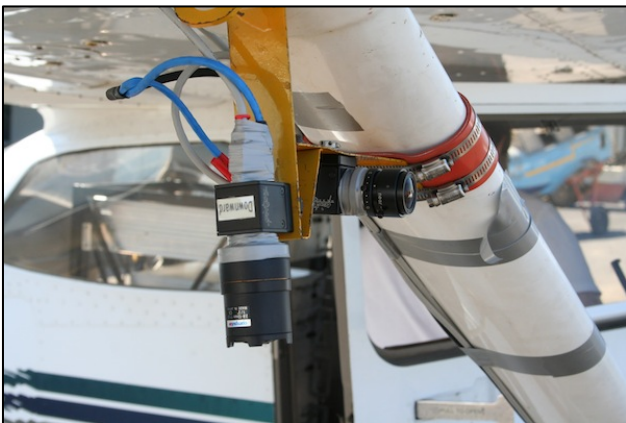
Figure 3: Dual camera system showing forward and downward pointing cameras.
