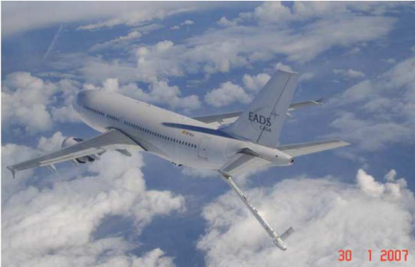
Fig. 2 Boom System in AIRBUS Military A310-Demo platform
