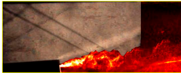
Fig.15. Overprinting of schlieren and NPLI images
