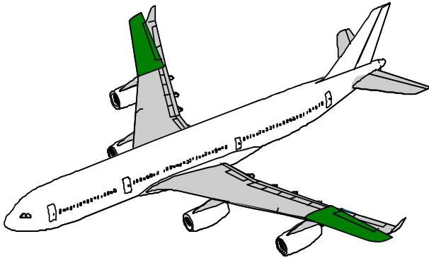
Fig. 1. Sketch of the “High Speed Demonstrator Passive” Airbus A340-300 Test Aircraft with “Smart Wing” Test Articles
