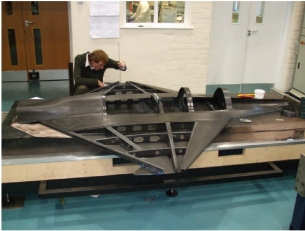
Fig. 5 Bonding of Composite Structures
