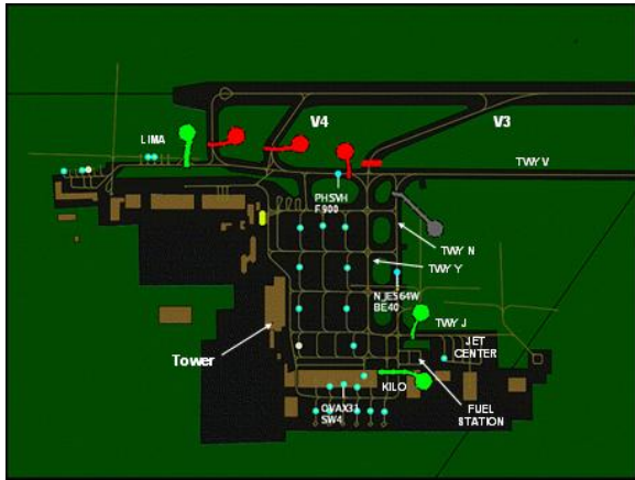
Fig. 1. Tower Controller radar screen with Virtual Bars (Green for pass, red for hold and grey for deactivated)
