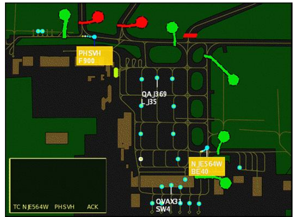
Fig. 2.b. Separation Bubble alert corresponding to the situation depicted in Fig. 2.a. The table specifies which aircraft cause the alarm.
