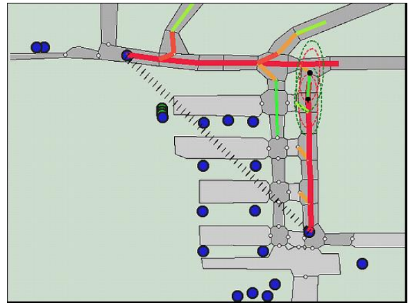
Fig. 2.a. Visualisation of the Separation Bubble algorithm with trajectory prediction of all theoretically possible routes. Blue dots are aircraft. Right:
