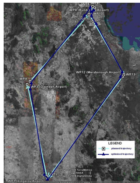
Fig. 9 Example Comparison of a Set of Optimised Waypoints (navy) for Minimum Fuel and Flight Time to the Baseline Flight Mission (light blue) (not to scale).
