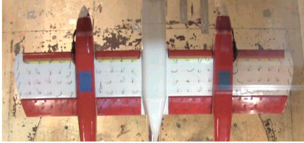
(c) \alpha = 24^\circ : completely separated flow
