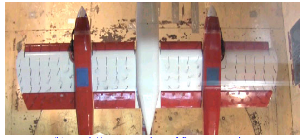
(b) \alpha = 24^\circ : progression of flow separation
