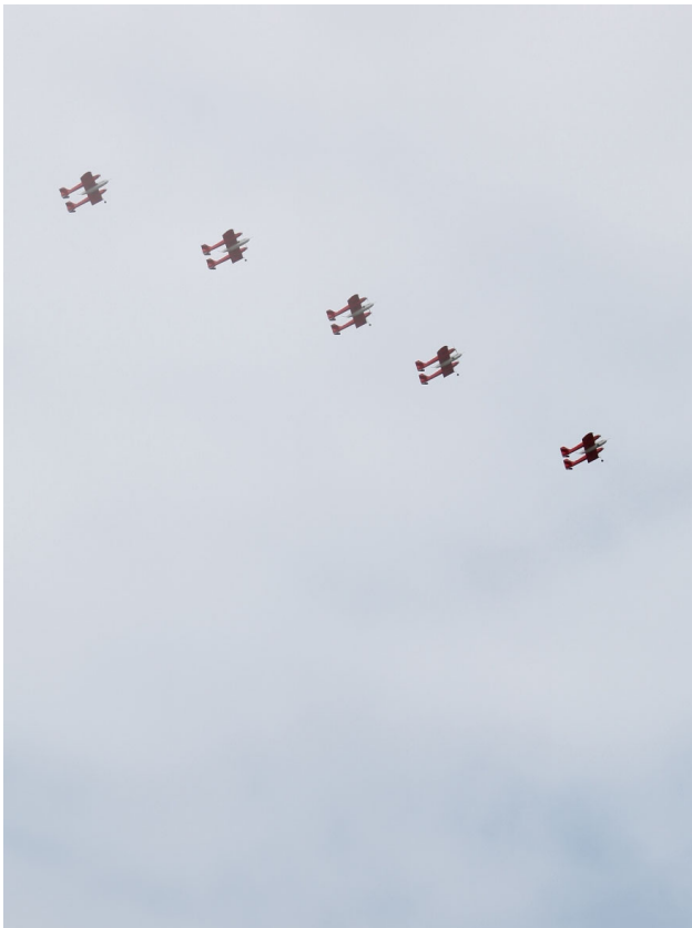
Fig. 12 Composite image obtained from a sequence of photographs of high AoA descent flight (wind condition: approx. 2.5 m/s windward, propeller rotation speed: 5500 rpm, photo shoot intervals: not constant (approx. from 0.5 to 0.75 sec))
