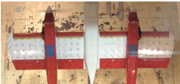
(c) \alpha = 30^\circ : completely separated flow
