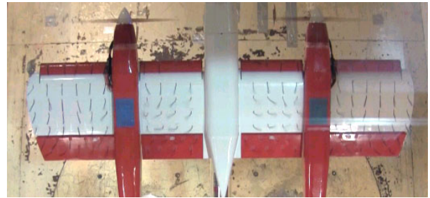
(b) \alpha = 24^\circ : flow separation limited to the inboard wing
