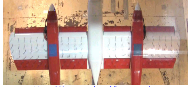
(c) \alpha = 30^\circ : progression of flow separation
