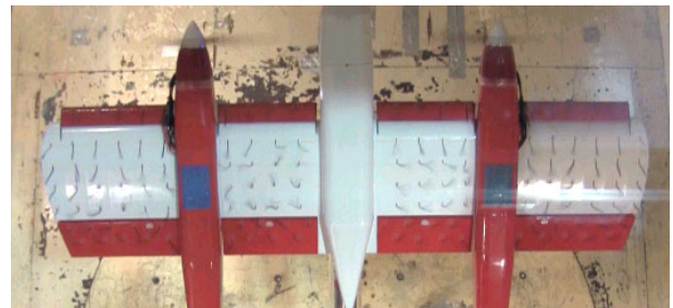
(c) \alpha = 30^\circ : flow separation progressed to the outboard wing
