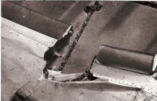
Fig.1. Bird strike damage of leading edge
