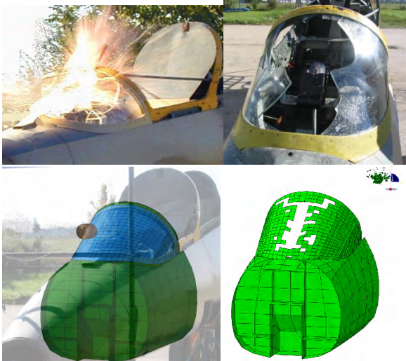
Fig.8. Result of test [3] (above) and FE simulation (below)
