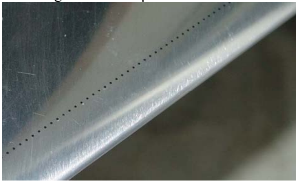
Fig. 4 Distributed roughness along the leading edge of the swept wing
