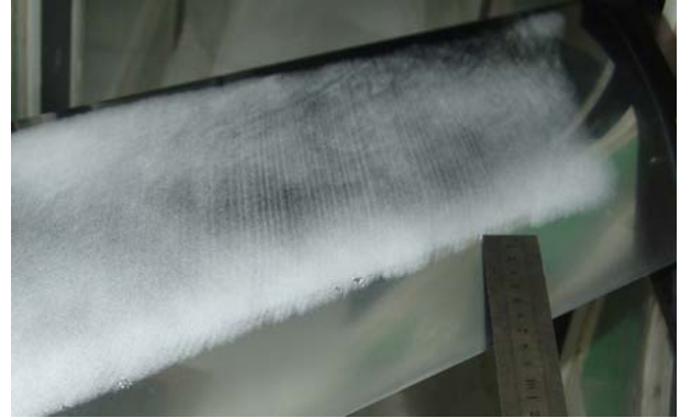
Fig. 10 Sublimation result without leading edge roughness at Re=1.38\times 10^6 in LTWT
