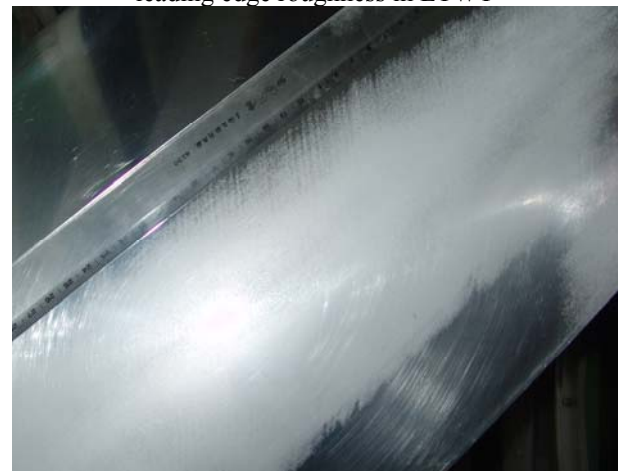
Fig. 20 Sublimation result at Re=1.38 \times 10^6 with 8.0mm leading edge roughness in LTWT
