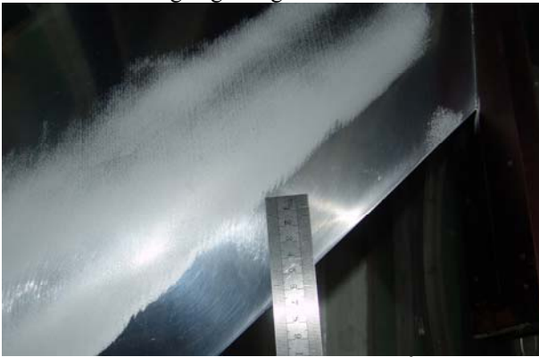
Fig. 17 Sublimation result at Re=1.38 \times 10^6 with 2.5mm leading edge roughness in LTWT
