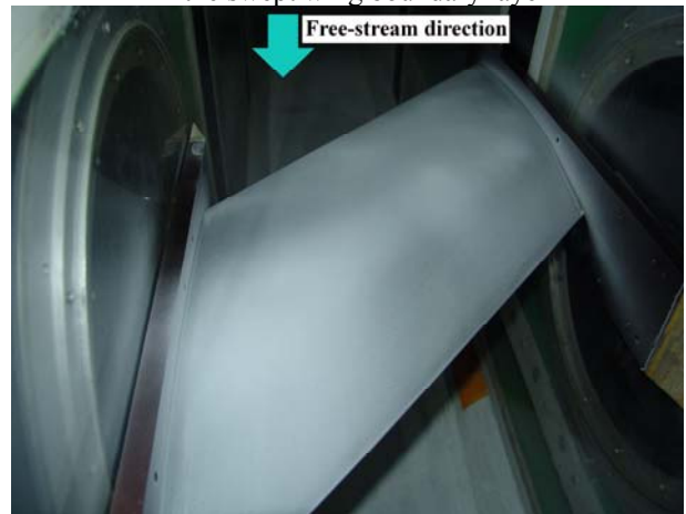
Fig. 6 Naphthalene sprayed on the entire upper surface of the model in LTWT
