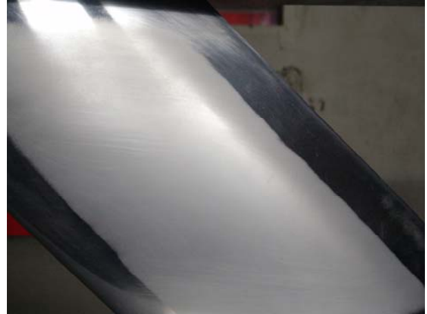
Fig. 23 Sublimation result without leading edge roughness at Re=1.38\times 10^6 in NF-3 wind tunnel
