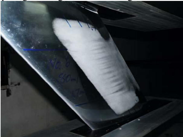
Fig. 26 Sublimation result at Re=2.20\times 10^6 with 1.7mm leading edge roughness in NF-3 wind tunnel
