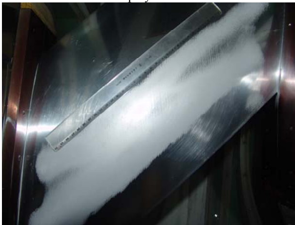
Fig. 14 Sublimation results at Re=1.65 \times 10^6 with the leading edge not sprayed in LTWT
