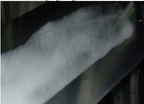
Fig. 18 Sublimation result at Re=1.38 \times 10^6 with 6.0mm leading edge roughness in LTWT
