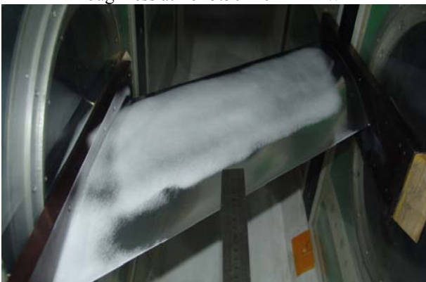
Fig. 9 Sublimation result without leading edge roughness at Re=1.10\times 10^6 in LTWT
