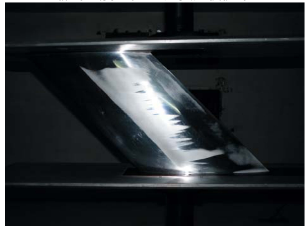
Fig. 24 Sublimation result without leading edge roughness at Re=2.20\times 10^6 in NF-3 wind tunnel
