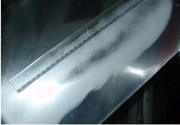
Fig. 16 Sublimation result at Re=1.10 \times 10^6 with 4.0mm leading edge roughness in LTWT
