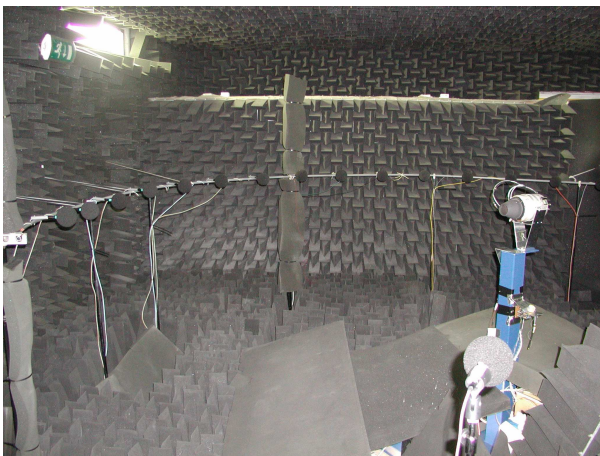
Fig. 4. Experimental set-up for stationary engine tests
