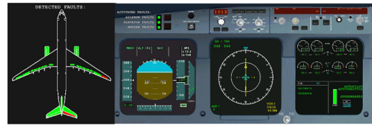
Fig. 6 2-D visualization of the fault status of A/C control surfaces
