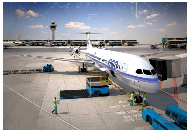
Fig. 1 Potential 2020 transport aircraft layout featuring a T-tail configuration and CROR in pusher configuration.
