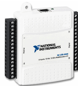
Fig. 9. A/D converter used to sample the recovered RSSI signal
