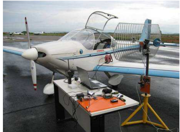
Fig. 17. Antenna pointer during the flight test
