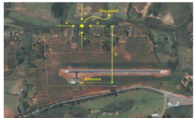
Fig. 20. Procedure for aircraft isotropy test
