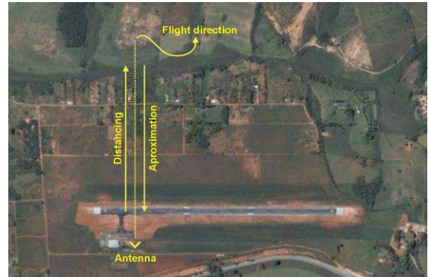
Fig. 22. Procedure for the signal strength measurement versus the distance
