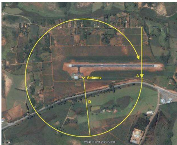
Fig. 21. Procedure for obtaining the radiation pattern of the antenna on the ground station
