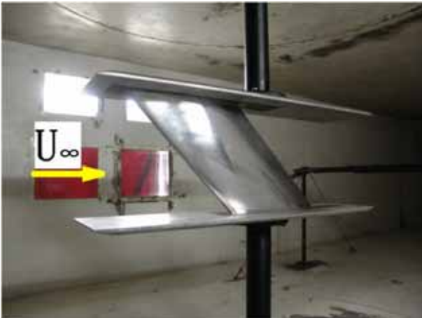
Fig.3. Model mounted in wind tunnel
