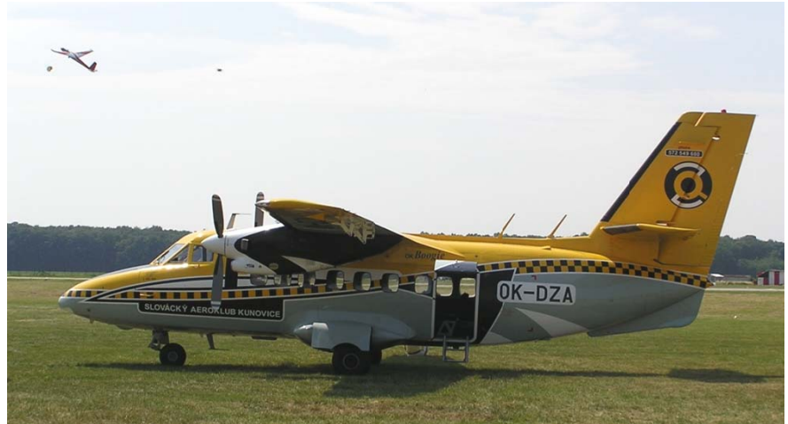
Fig. 7. L-410 aircraft (2-engine turboprop, 19-seats)
