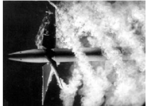
Fig. 8. Single propeller swirl
