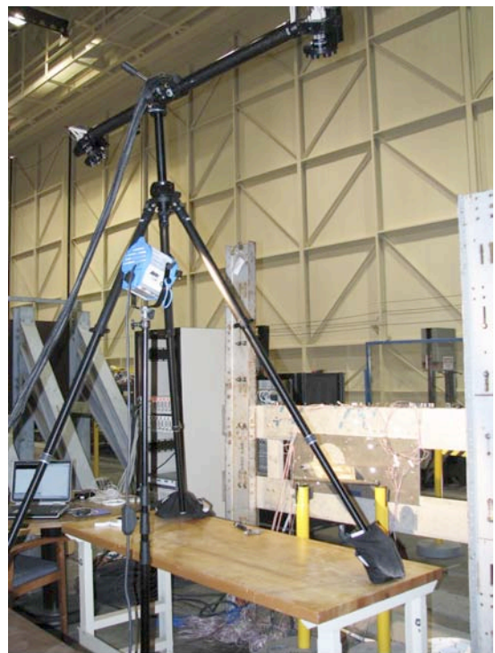
Fig. 6. The PONTOS photogrammetry optical measuring system.
