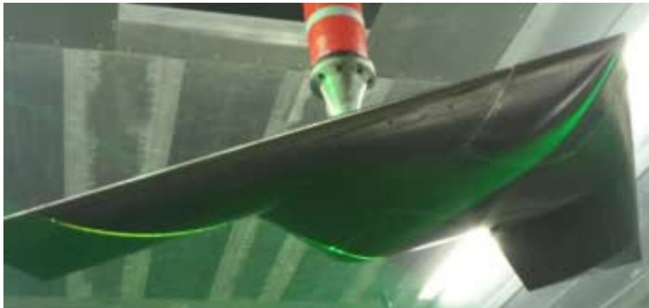
Fig. 4 MODEL MOUNTED (UPSIDE-DOWN), DNW LOW-SPEED WIND-TUNNEL
