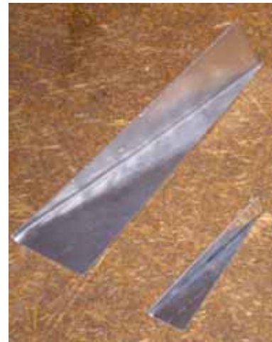
Conventional VG (left) and Micro-VG (right).
