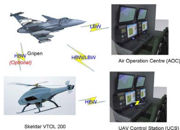
Figure 2. Example of actors in the CAS scenario: A manned A/C, UAV and ground control stations (AOC + UCS). HBW=High Bandwidth, LBW=Low Bandwidth
