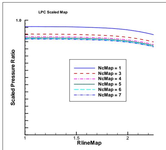
Figure 4b. LPC component map using a scaled map. Displayed is the scaled pressure ratio across the component versus the rotor operating speed. The index indicates the convergence history of the maps with the 7th iteration resulting in a full multi-level convergence.
