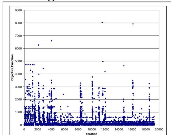
**Figure 3. Optimization output of the AXOD matching process. Minimizing the objective function provides the best match between high-fidelity and cycle maps.**
