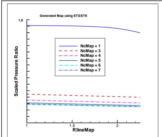
Figure 4a. LPC component map using a generated map from STGSTK.
