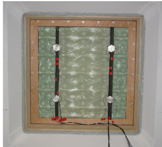
Fig. 15: Fuselage panel with active attachment elements installed to the frames
