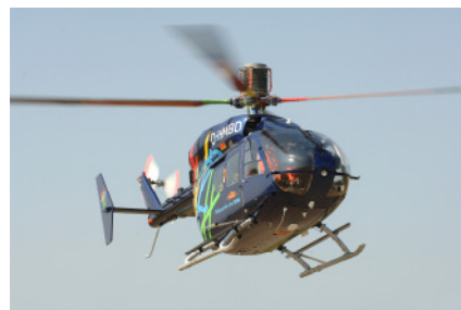
Fig. 4: BK117 S7045 with active flaps rotor
