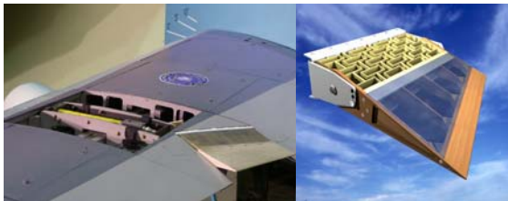
Fig. 12. Adaptive inner aileron; compartment 3-component strain gage balance; SDS prime structure (without elastomeric filler)
