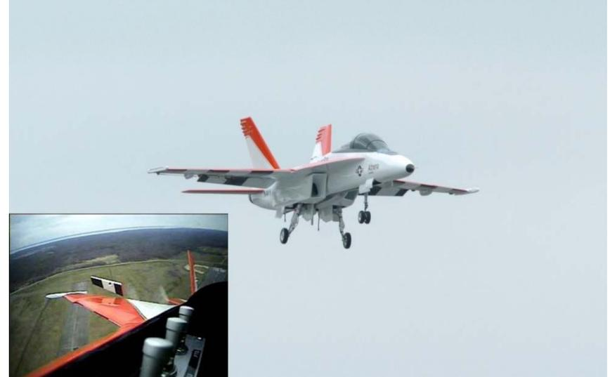
Inset: Ejected aileron simulating battle damage
