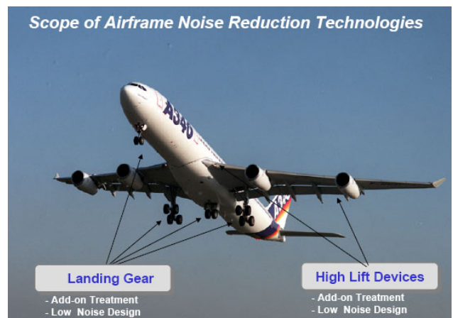
Fig. 6: The SILENCE project used the A340 SN 001 for airframe noise reduction research (Source: SILENCE(R)/ SNECMA)
