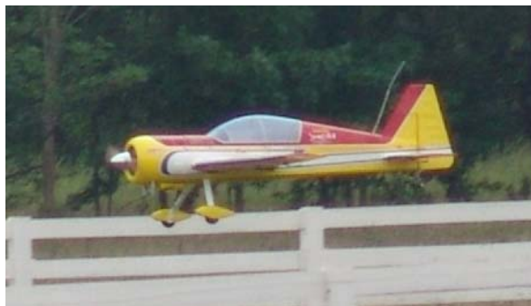
Figure 7: Follower aircraft #2 for flight test, able to maneuver similar to leader, includes onboard cameras and image processing, estimation, and guidance computer
