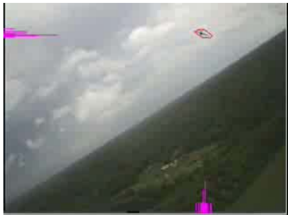
Figure 2: Tracking aerial targets against clutter using particle filtering, horizontal and vertical distributions of target location probability density (from particle filter) shown on edges.
