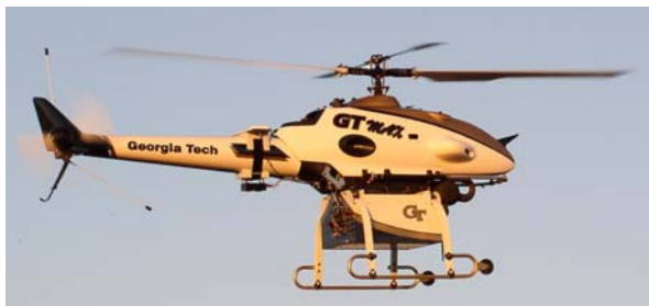
Figure 6: Follower aircraft #1 for flight tests, a 10 ft rotor diameter helicopter, includes onboard cameras and image processing, estimation, and guidance computer
