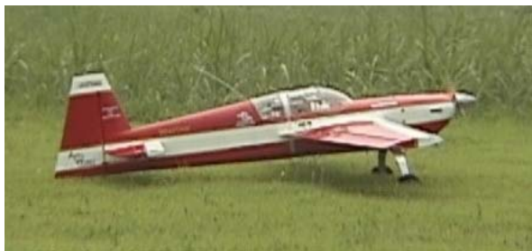
Figure 5: Leader/target aircraft for flight tests, at 9 ft wing span airplane
