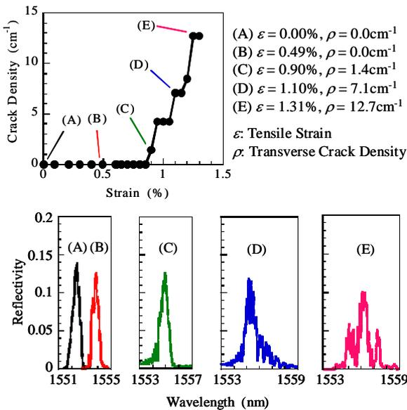
Fig. 5: Change in wavelength distribution of reflected light from the FBG sensor due to the evolution of transverse cracks.
