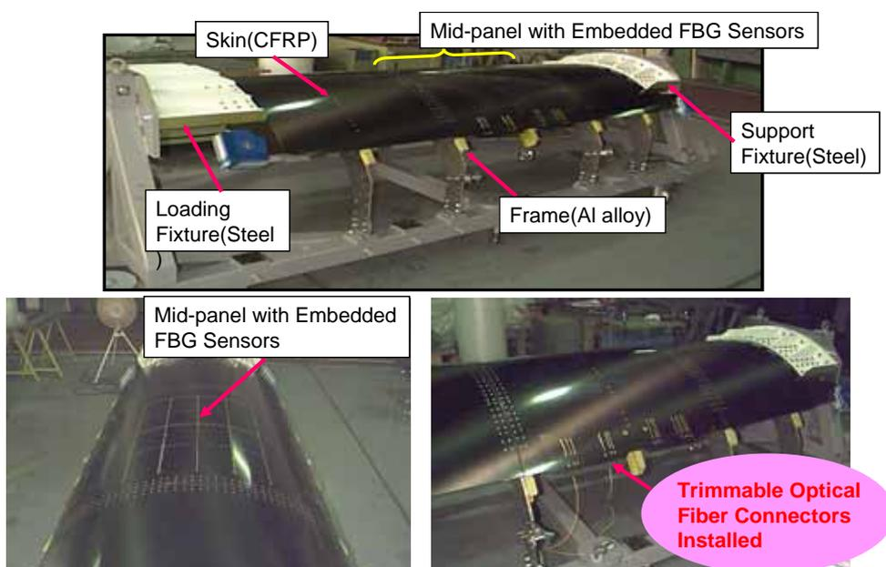
Fig. 12. Upper panel with embedded small-diameter optical fibers and trimmable connectors.
