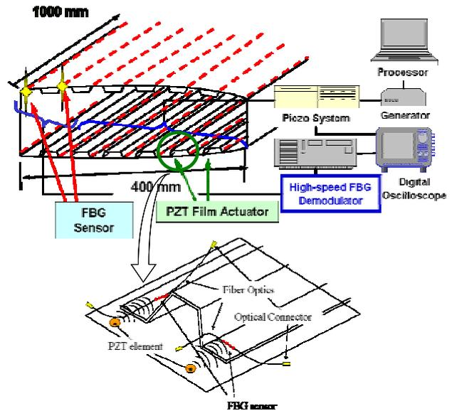
Fig. 15. Lamb wave detection in CFRP box structures with high-speed optical wavelength interrogation system using an AWG filter
