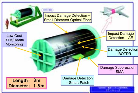
Fig. 9. Selected themes in Damage Detection and Suppression Demonstrator Test
