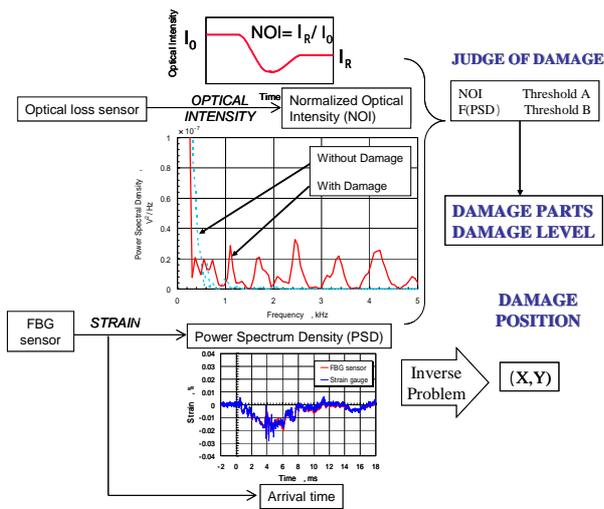
Fig. 13 Algorithm of impact load and damage evaluation/visualization system
