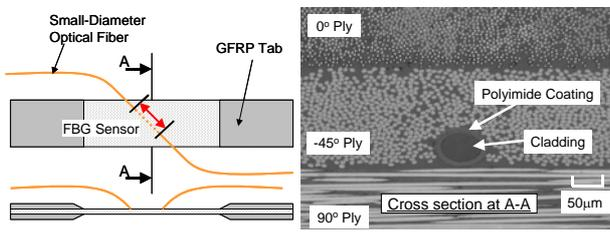
Fig. 4. A small-diameter FBG sensor embedded in the  $-45^\circ$  ply for detection of transverse cracks in the adjacent  $90^\circ$  ply of quasi-isotropic  $[45/0/-45/90]_s$  laminate.
