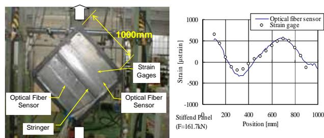
Fig. 21. Comparison of strain distribution between BOCDA and electrical strain gages in buckling tests of stiffened panels.
