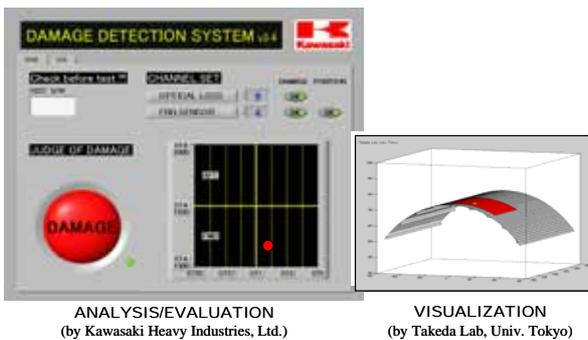
Fig. 14. A developed impact detection and localization system. The system judged a delamination at the impact region.
