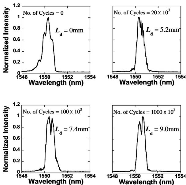
Fig. 7. Change in wavelength distribution of reflected light from the FBG sensor due to the edge delamination growth.
