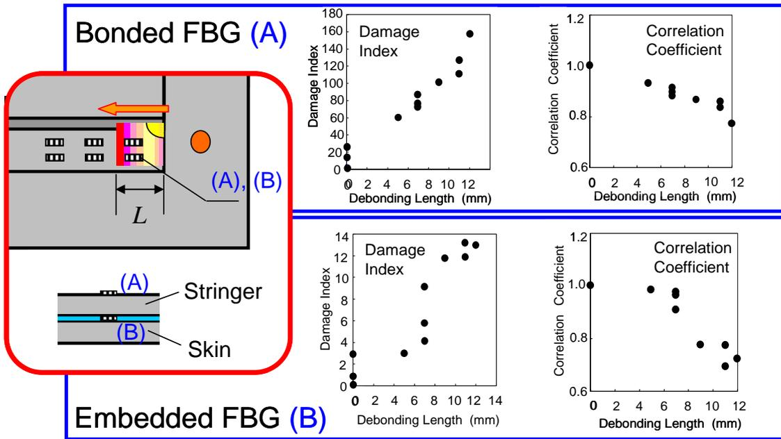
Fig. 18. Damage index  $DI$  and correlation coefficient  $c$  as functions of debonding length.
