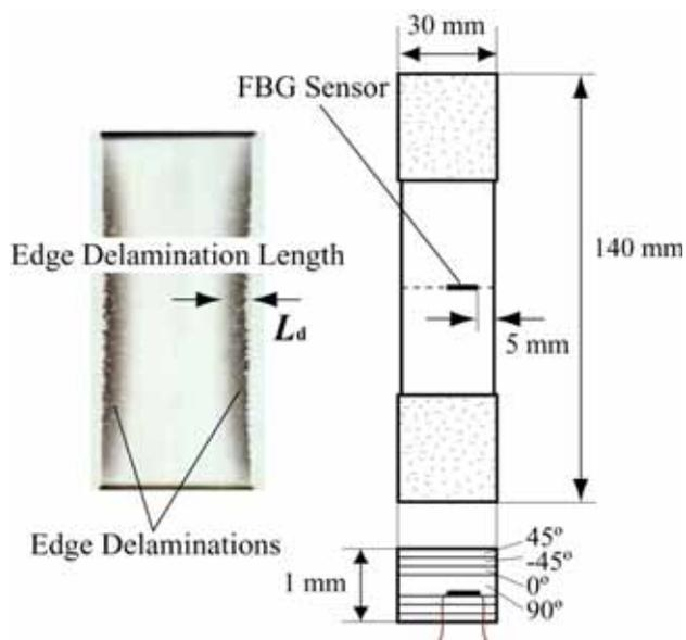
Fig. 6. Schematic of  $[45/-45/0/90]_s$  edge delamination specimen with an embedded FBG sensor.
