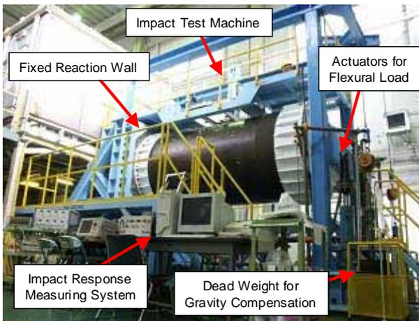
Fig. 8. Final assembly of the Damage Detection and Suppression Demonstrator
