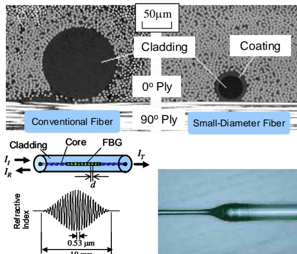
Fig. 2. Conventional and small-diameter optical fibers embedded in a CFRP lamina and small-diameter FBG sensors with fiber connection to conventional optical fibers.
