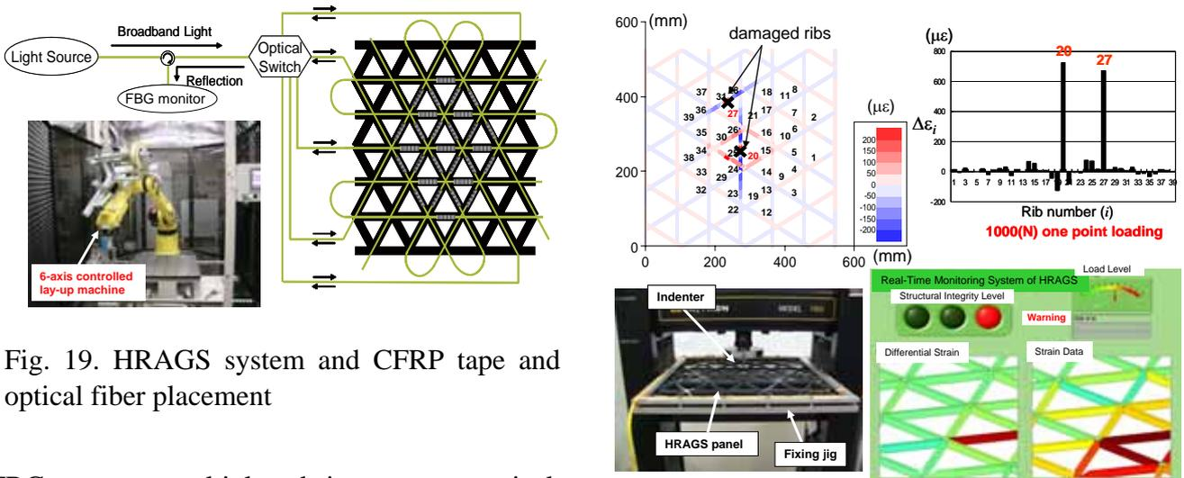
Fig. 19. HRAGS system and CFRP tape and optical fiber placement
