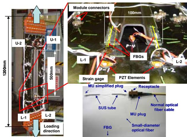
Fig. 16. Fatigue test of a CFRP box structure with the hybrid and active sensing system. Pre-installed optical connectors were installed.
