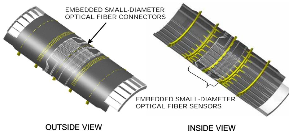
Fig. 11 Schematic of arrangement of embedded small-diameter optical fibers in the upper panel.
