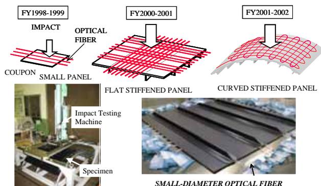
Fig. 10. Impact test specimens from coupons to stiffened flat and curved panels with embedded small-diameter optical fibers
