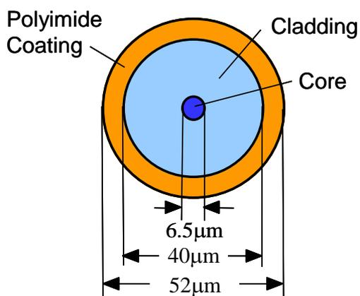
Fig. 1. Small-diameter optical fiber
