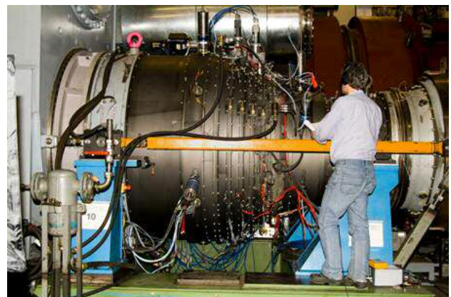
FIG. 14: High Lift rig installed in ATF in Stuttgart
