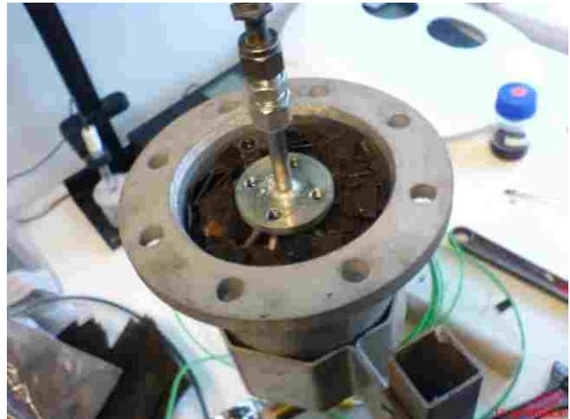
Picture 7. Assembling of the full scale gas generator.
