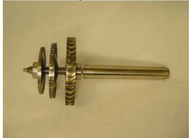
Picture 1. The Atlas Copco turbine rotor
