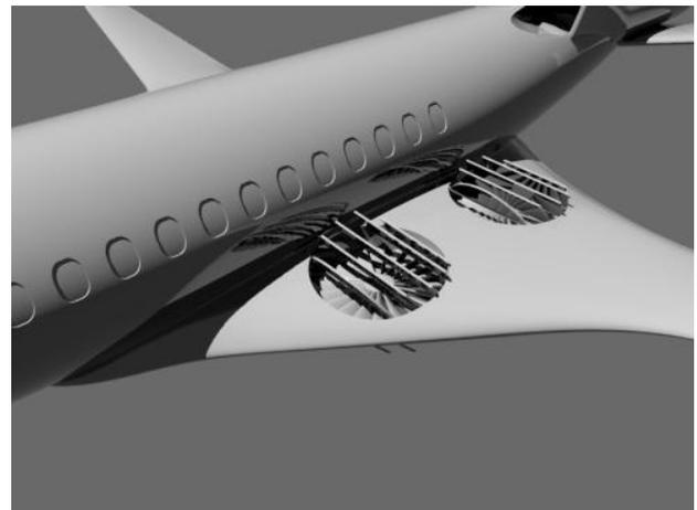
Fig. 5 Lift-fan integration
