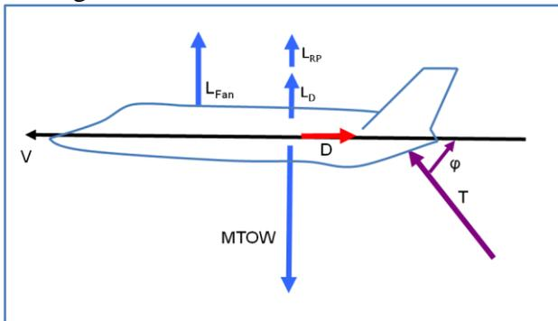
Fig. 1 Forces acting during take off and landing
