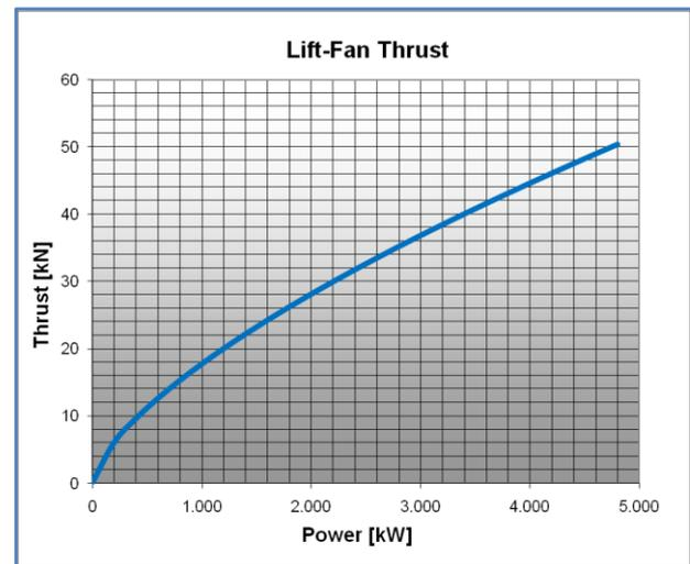
Fig. 10 Lift-fan thrust over available power
