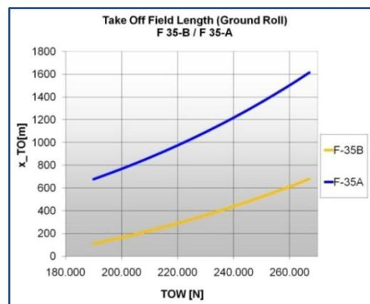
Fig. 2 Calculated Take Off Field Length for JSF
