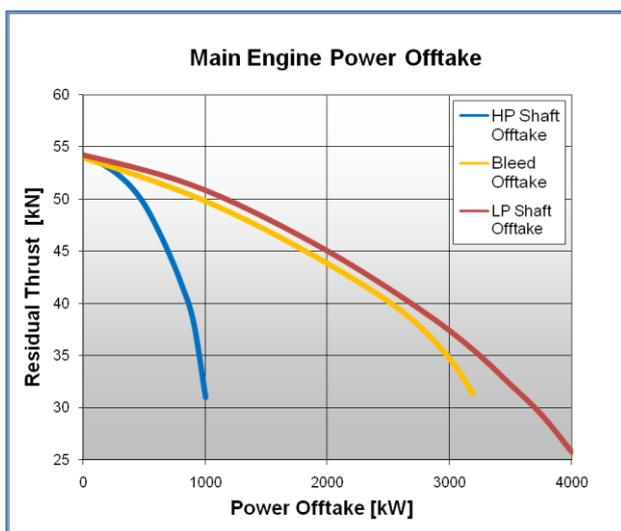
Fig. 9 Residual thrust over power offtake
