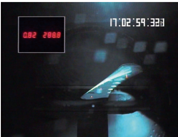
Fig. 10 Image of CCD camera (the wing without engine nacelle model)
