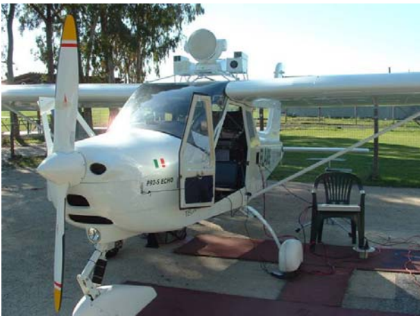
Fig. 3. Obstacle detection sensors mounted on-board FLARE
