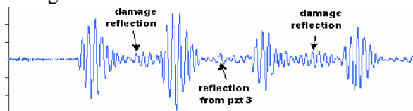
Fig. 16. Identification of damage reflections
