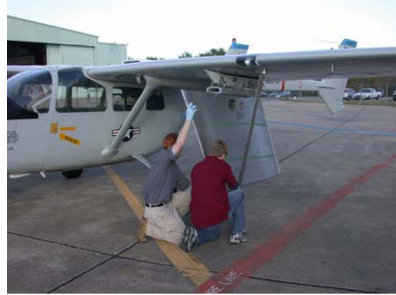
Fig. 6. O-2 Skymaster with the SWIFT model attached beneath the port wing.
