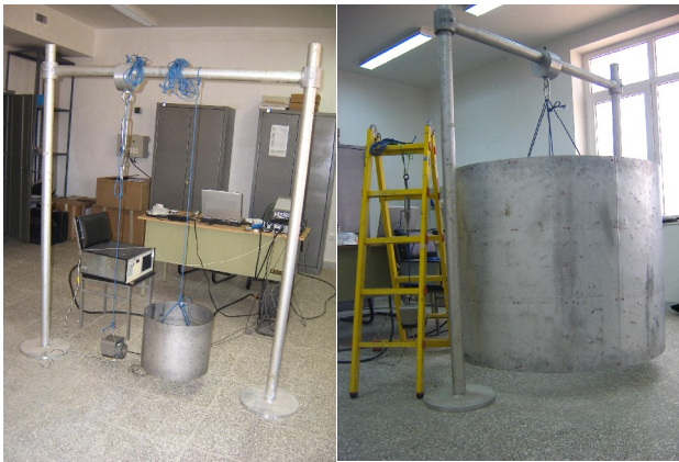
a) Modal testing of the model b) Modal testing of the prototype
