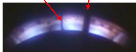
(c) Photo image of traverse measurement in combustion test under 7% MTO condition.
