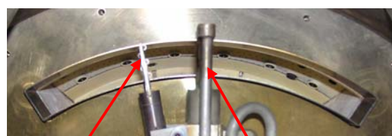
(b) Temperature sensor rake and gas sampling probe traverse measurement system at combustor exit.
