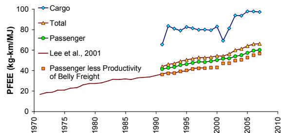
Figure 8: Comparison of data from [1] with the historical fleet-wide PFEE data from Figure 7.
