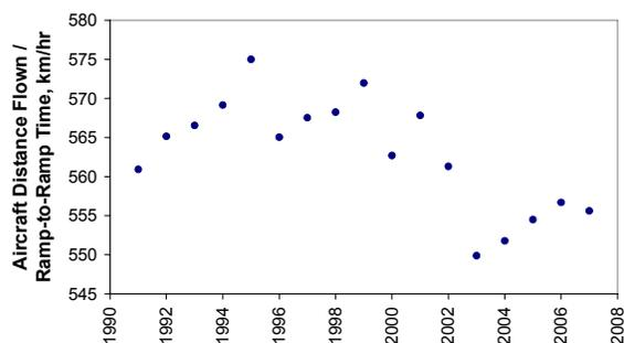
Figure 6: Effective cruise speeds for U.S. carriers (data from [9]).
