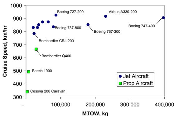
Figure 5: Typical cruise speeds for select aircraft, as reported by the manufacturers.
