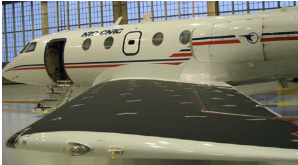
Figure 6: Photograph of the Falcon aircraft with the left wing painted black and covered with tufts for flow visualization. The IR camera is located behind the emergency exit door.
