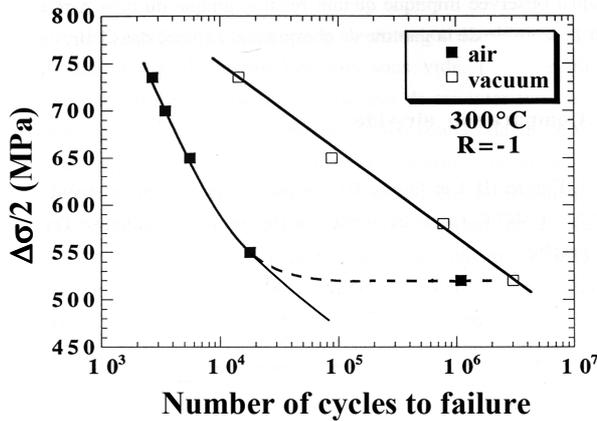
**Fig. 1** S-N curve, Titanium Ti 6246 alloy at 300°C, load ratio  $R = -1$ , under vacuum and air environment.
