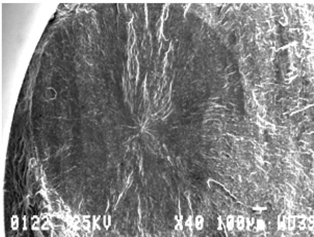
**Fig. 2** Fracture surface (SEM observation) of Ti 6246 : internal initiation.
