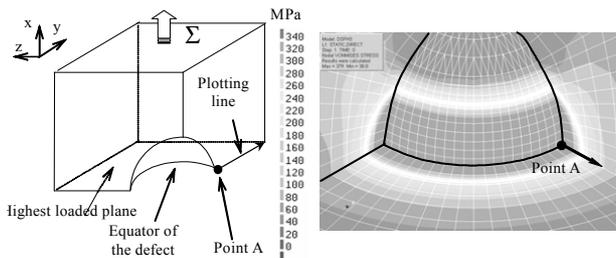
**Fig. 7.** Details of the geometry and the mesh under tension
