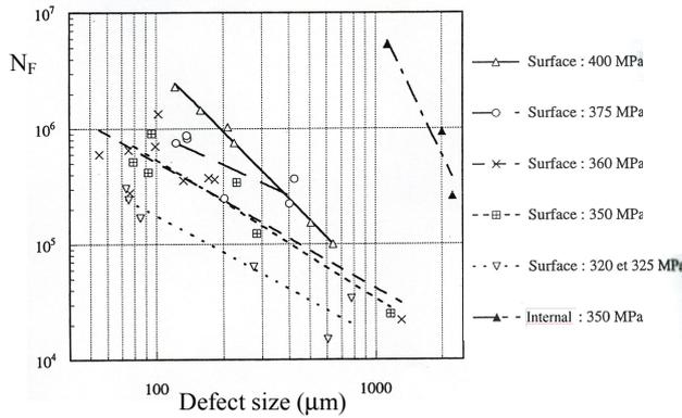
**Fig. 5** Evolution of the number of cycles to failure for different stresses versus defect size,  $R = 0.1$
