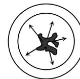
**Fig. 3** Fracture surface (SEM observation) of nodular cast iron: internal initiation.
