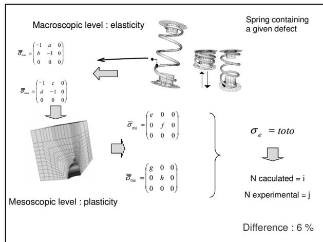
**Fig. 8.** Application of the criterion to suspension spring containing a surface defect
