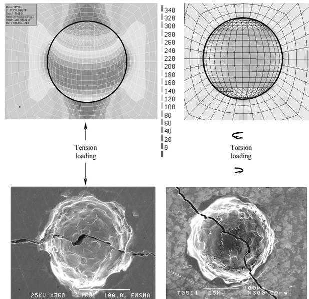
**Fig. 6.** Stress state (von Mises equivalent stress) around a spherical defect under tension and torsion and corresponding crack path from SEM pictures.
