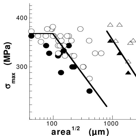
**Fig. 4** Evolution of the fatigue limit with defect size for both surface an internal defect,  $R = 0.1$
